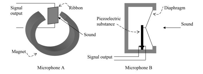
**Question 7** Identify the two types of microphones as dynamics, crystal, velocity or electret-condenser. Briefly explain the working of each microphone.
