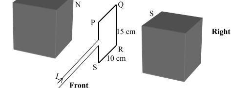
A rectangular loop PQRS (15 cm by 10 cm) of 20 turns of insulated copper wire is placed between two opposite magnetic poles as shown in the diagram above. It shows the initial orientation of the loop. There is an electric current I = 2.0 A in the loop. The magnetic field is uniform B = 0.5 T between the poles.
